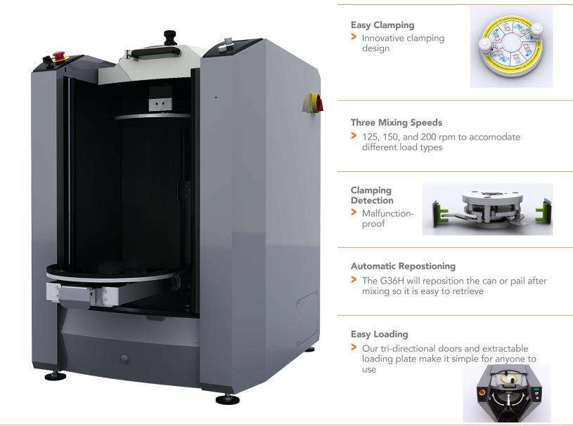
G36 Manual Clamping Mixer Shaking Mode Gyroscopic Mixing Volume Quart to Five Gallons Max Mixing Weight 79 lbs Mixing Time 30-900s, in 30s increments Mixing Speed 125/150/200 rpm Smallest Can Size 2x3.5" Largest Can Size 14x15.75" Direct Shipment 20 pcs per 20GP Power 350W Power Supply 110V 60Hz Machine Dimension (WDH) 31x34x42" Shipping Dimension (WDH) 37x33x47" Net Weight 508 lbs Shipping Weight 563 lbs
